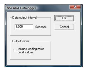
This dialog allows the Data output interval for the NORCOM Datalogger to be changed, from the default value of 1 second to the appropriate interval. It also allows the operator to include leading zeros on all output fields effectively making the telegram a fixed field fixed length telegram.
